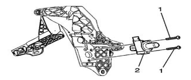
Fig. 15: View Of Accelerator Actuator & Actuator Mounting Screws Courtesy of GENERAL MOTORS CORP.
