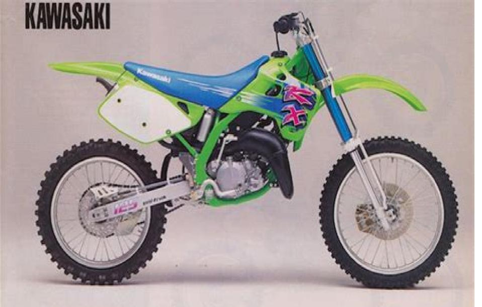
Changes to the KX125 and 250 start with a new frame and plastic. The upper shock mount has been changed (doing away with the bolton triangles) and the midsection is silimmer. A lower tank is completely enclosed by the radiator shrouds and the pipe is lower. The silencer is also new. Overall, the bikes look much more sleek, don't you think?
