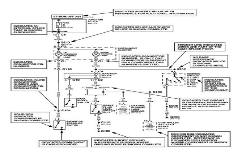
The System shown here is an EXAMPLE ONLY. It does not represent the actual circuit shown in the WIRING DIAGRAM SECTION.
