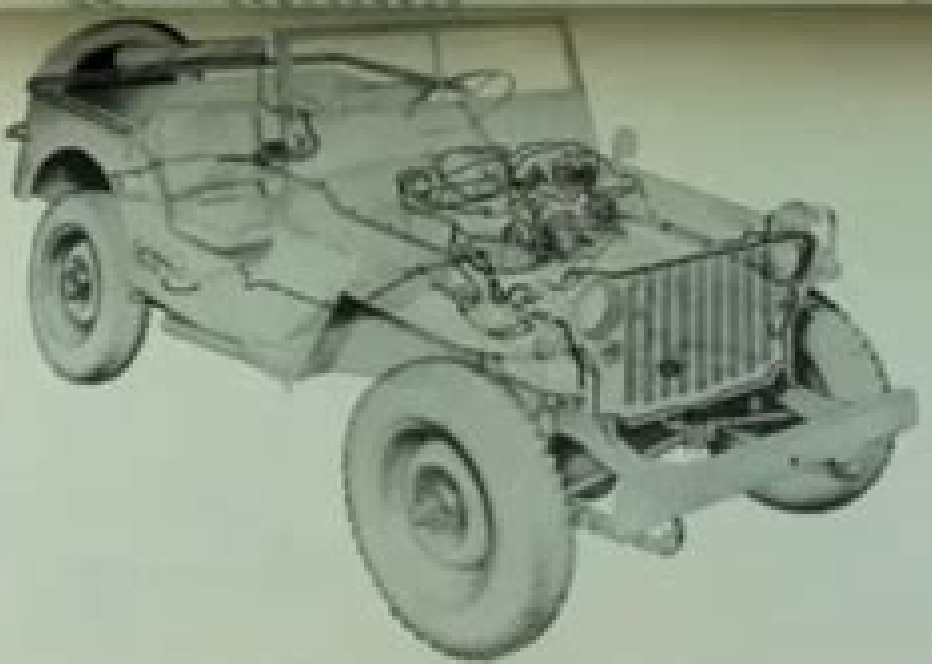
Figure 50—Wiring System—Phantom View
