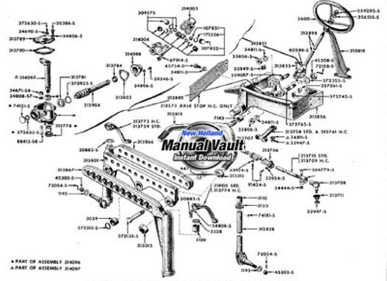
FIG. 3A3 - FRONT SUSPENSION, STEERING SYSTEM & RELATED PARTS
