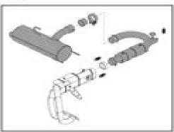
NOTE: The exhaust silencer can be removed through the side of the vehicle after the exhaust pipe is detached from the header pipe.
