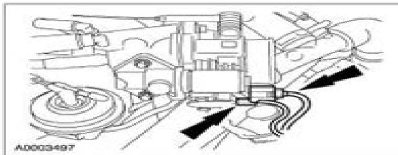
6. Disconnect the accelerator and speed control cables.
