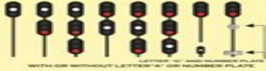
RULE 245M RESTRICTING Proceed at restricted speed, not exceeding prescribed speed through turnout.
